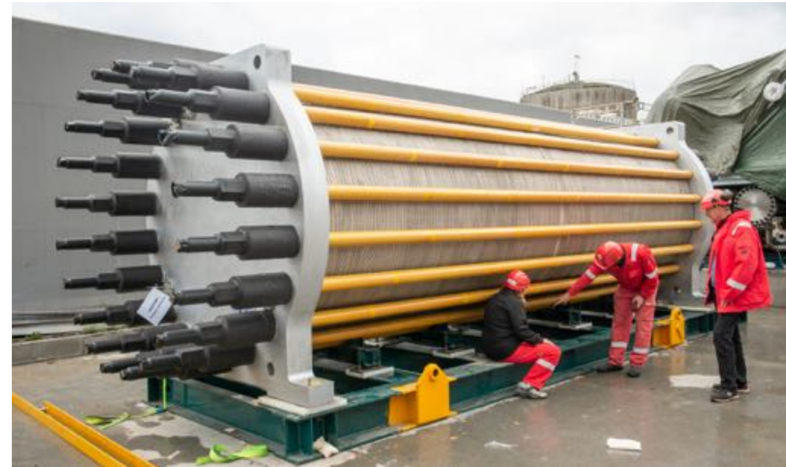
HydrogenPro taking delivery of the world's largest electrolyser at its test facilities in Herøya, Norway. Image courtesy HydrogenPro, September 2022.
